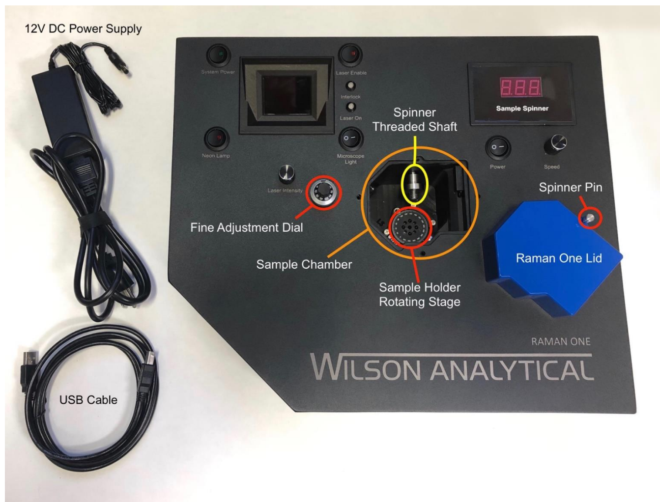
Figure 1. Raman One parts identification. Sampling accessories are sold separately.
