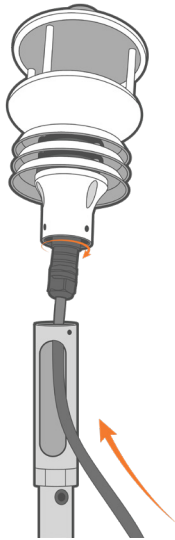
Figure 4: Connect the MaxiMet sensor cable.
