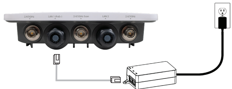
Access Point connected to PoE+ injector
