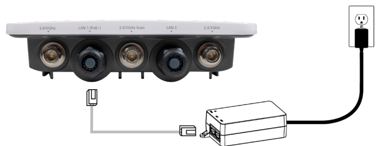
Access Point connected to PoE+ injector
