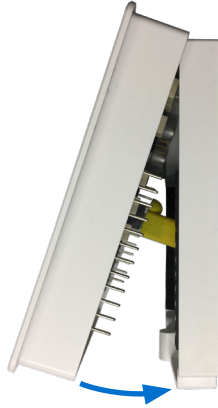
Illustration 7—Reinstalling the Cover on the Backplate
