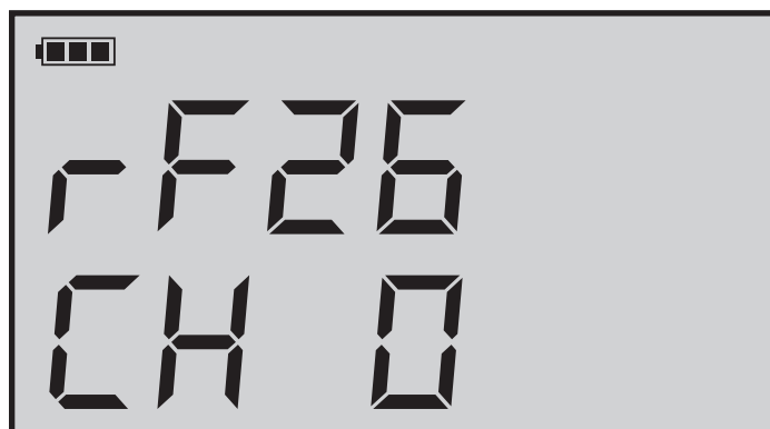
Figure - 4: Count down to connect with the scale platform on channel 0.
