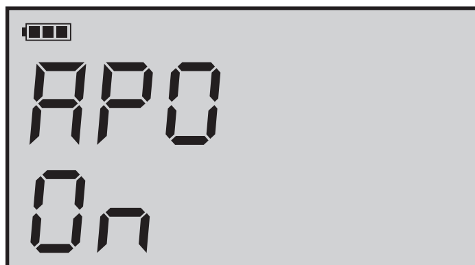
Figure - 6: Scale platform Automatic Power Off status.
