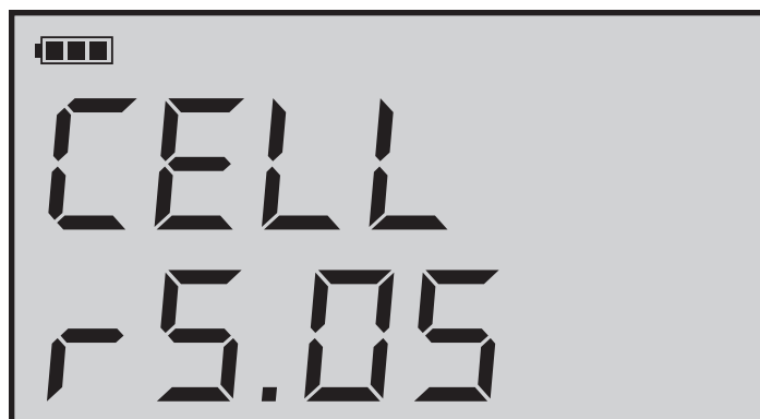
Figure - 7: Scale platform battery voltage.
