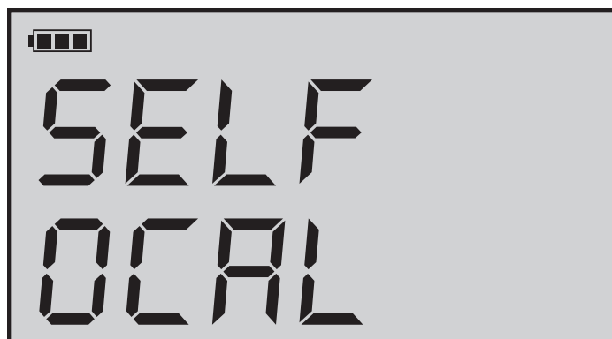
Figure - 8: Notifies the user that a zero calibration is being performed.
