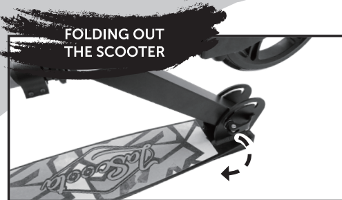
Open the quick-release lever.
