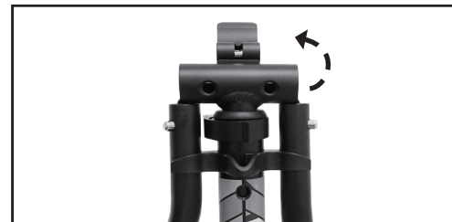
Open the handle bar clamp.
