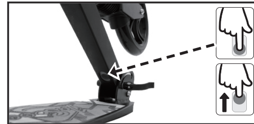
Open the handle bar clamp.
