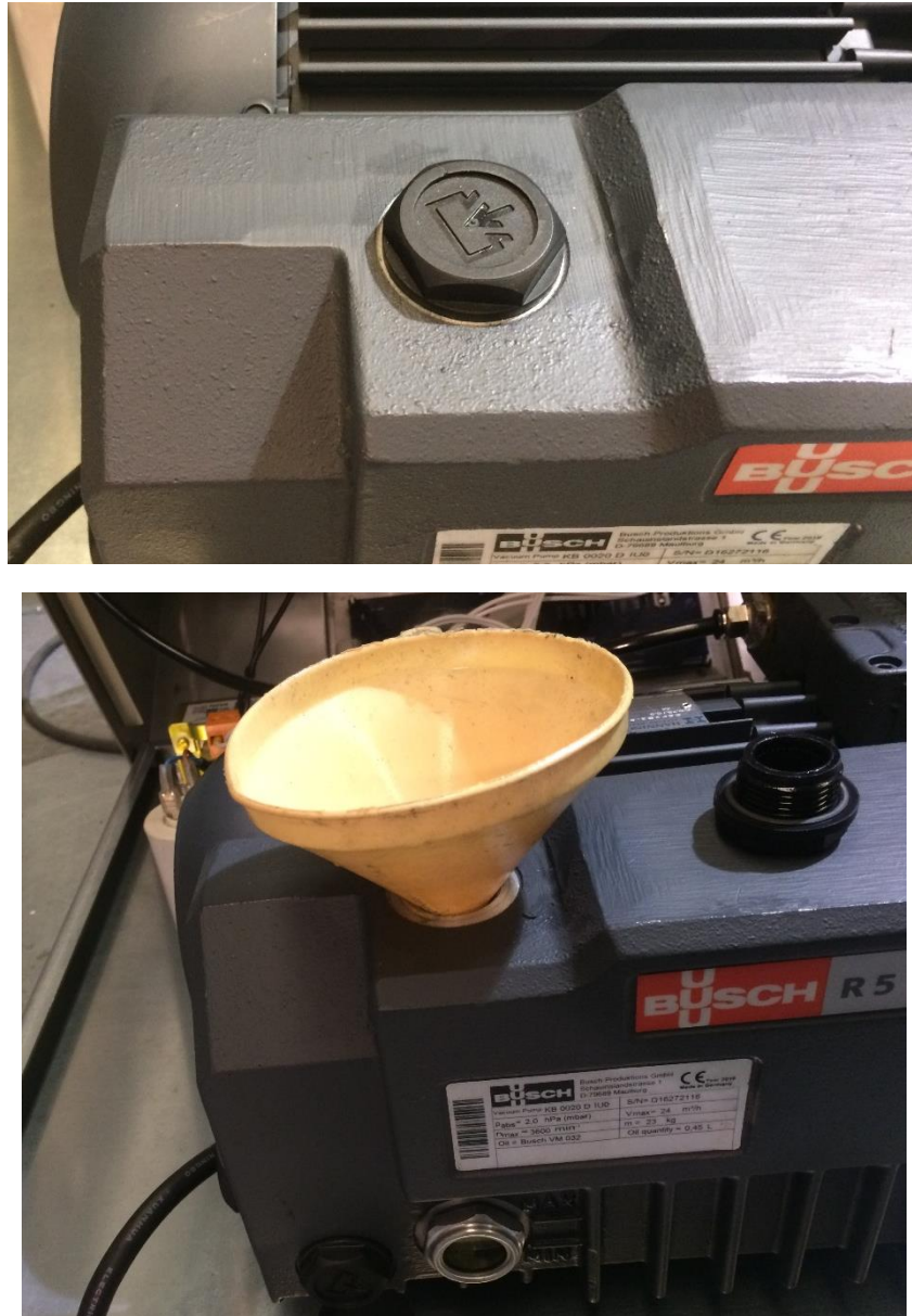
Illustration 7. Remove the oil filling plug and refill with new oil
