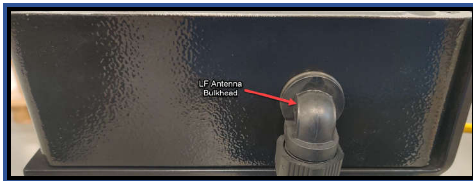
LF Antenna Bulkhead
