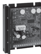
Brushless DC Drives Closed loop accuracy, line and low voltage versions through 1 HP
