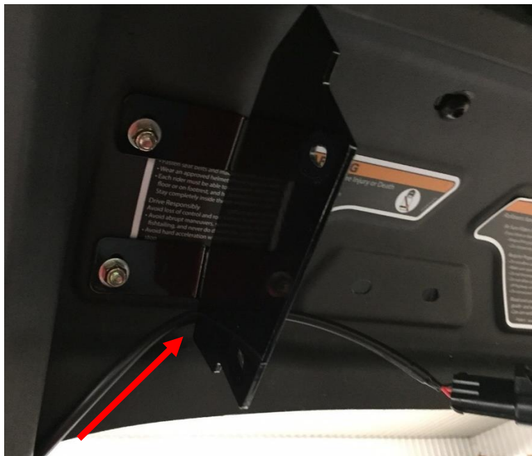
Figure 16: Placement of the chassis harness connector before mounting the unit.
