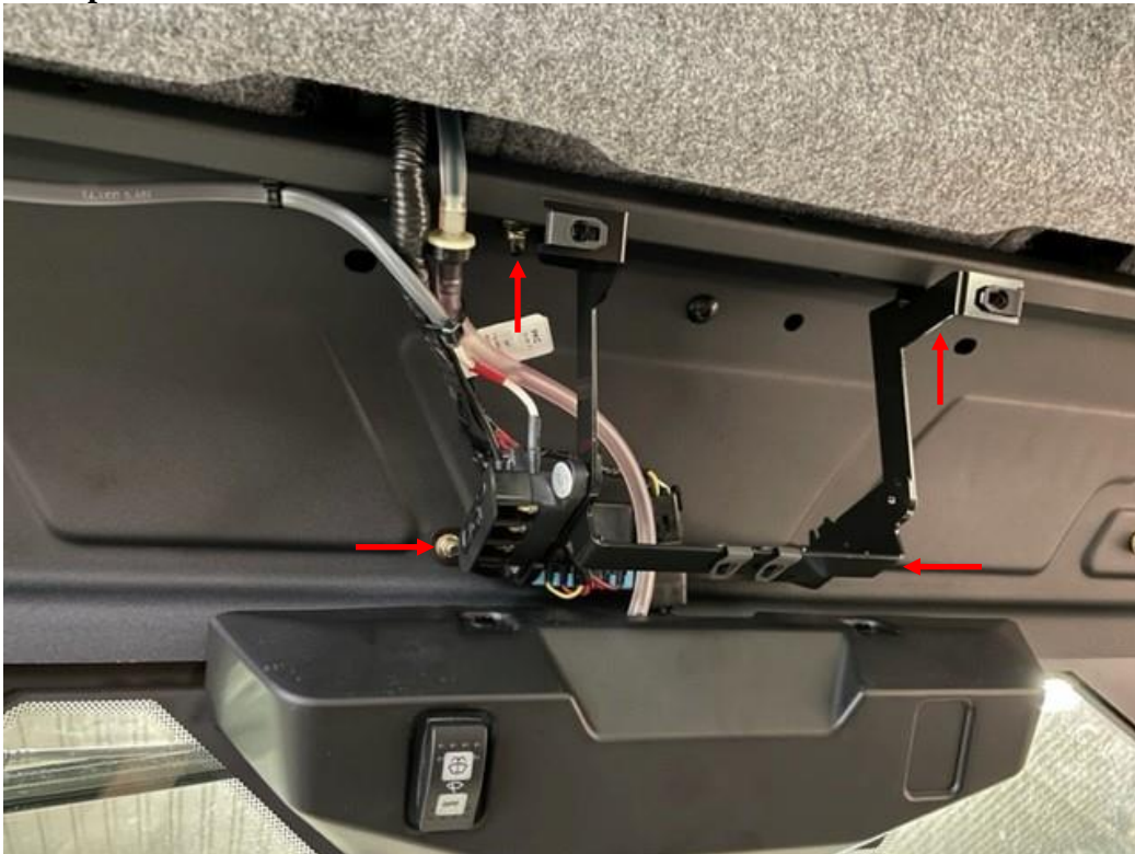
Figure 10: Remove the center roof liner bracket.
