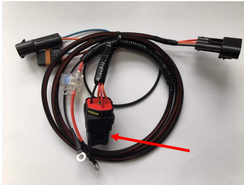
Figure 2: Chassis harness ignition relay
