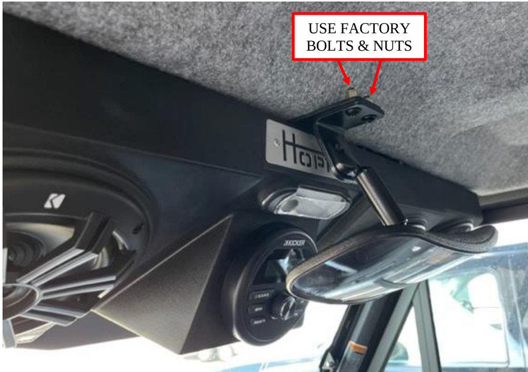
Figure 23: Mount the rearview mirror on the bracket.
