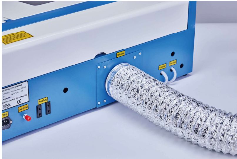
Fig. 2–2. The exhaust pipe connected to the rear of the engraver.
