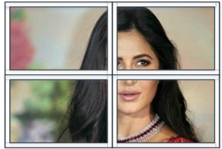
Correct Bezel Compensation
