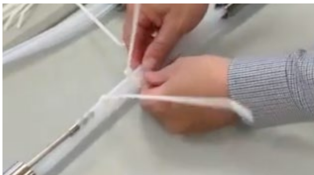
Keep tubing from twisting before adding extension.
