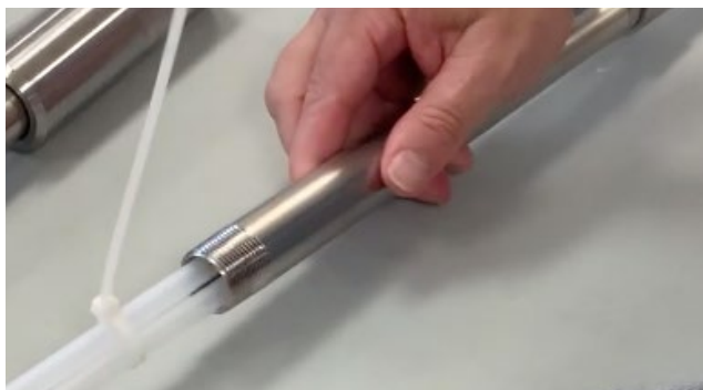
Push/move the cable tie along to keep tubing grouped and avoid twisting.
