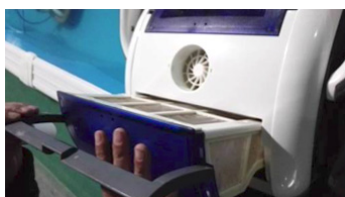
7. Slide the filter tray along the groove
