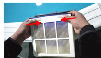
3. Push towards the middle to open the filter tray
