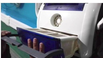
7. Skyv filterplaten tilbake i bassengroboten langs sporet
