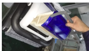
2. Lift the filter tray
