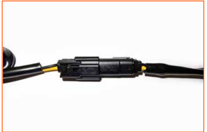
MAIN RADIO TO BATTERY HARNESS
