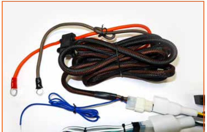
AMPLIFIER INPUT POWER CONNECTION
