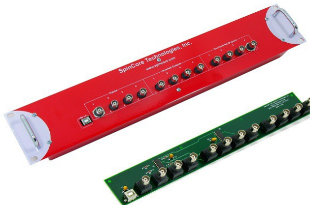
Figure 18: TTL Line Driver assures TTL levels over 50 Ohm loads.
