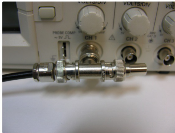
Figure 10: BNC T-Adapter on the oscilloscope with coaxial transmission line connected on the left and BNC 50 Ohm resistor connected on the right, to terminate the line.
