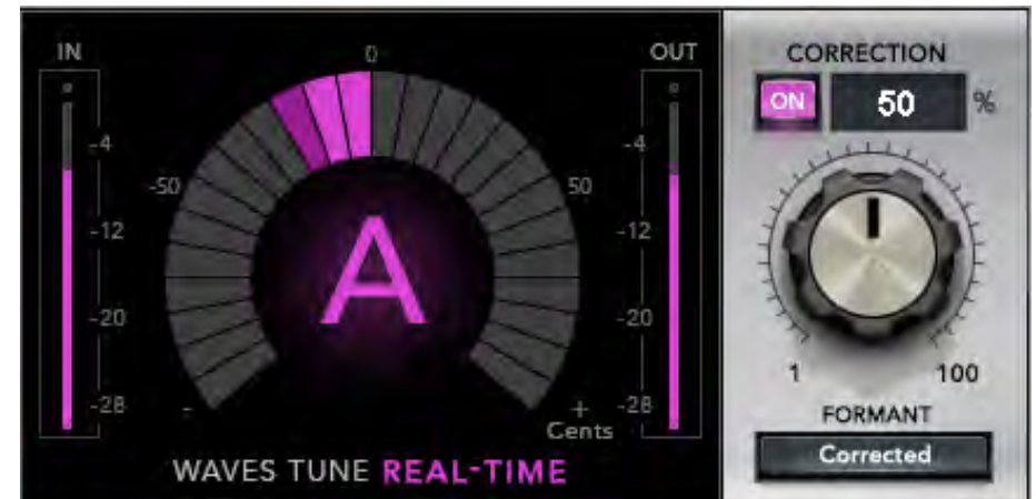
Example 2: Correction knob is set to 50%. The meter shows 20 cents pitch down.
