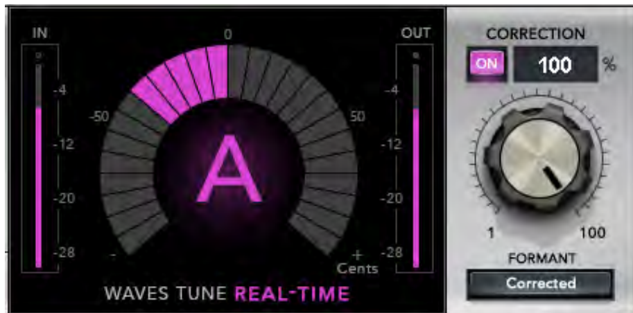
Example 1: Correction knob is set to 100%. The meter shows 40 cents pitch down.
