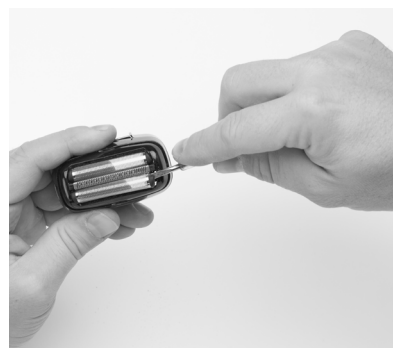
FIG. 3 USING A SMALL BLADE OR SCREWDRIVER, CAREFULLY LIFT OUT THE FOILS FROM THE SIDE, ONE AT A TIME [FIG. 3-4].
