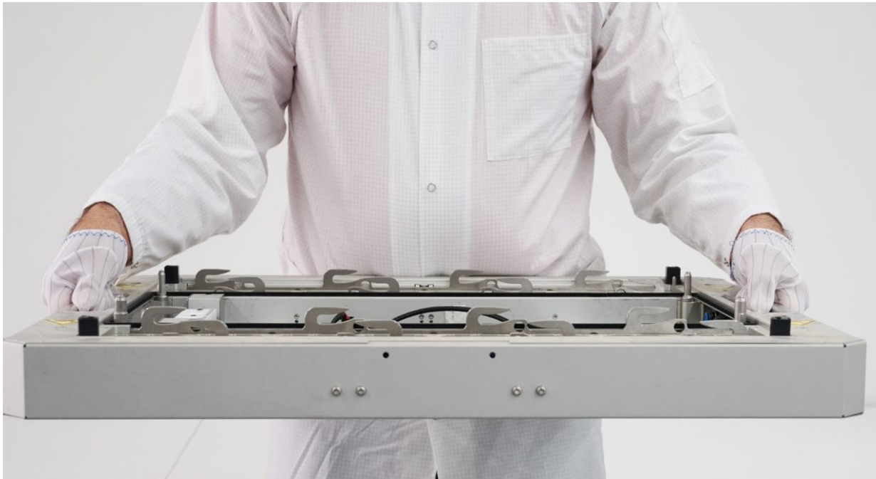
Figure 6: Multilane Card Cage (aka "Twinning Frame")
