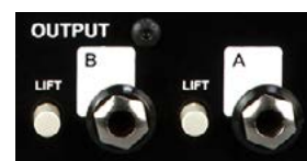
The amp outputs and lift switches
