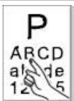
The toner does not adhere to the paper
