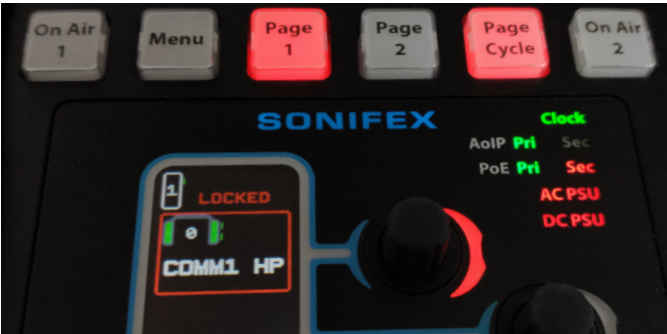
Fig 6-40: Locked user button warning
