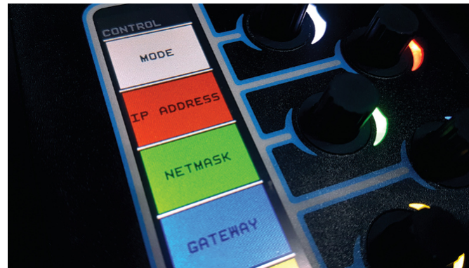
14. This sub-menu shows the IP address settings of the control port, select 'IP Address' by pressing the red encoder.
