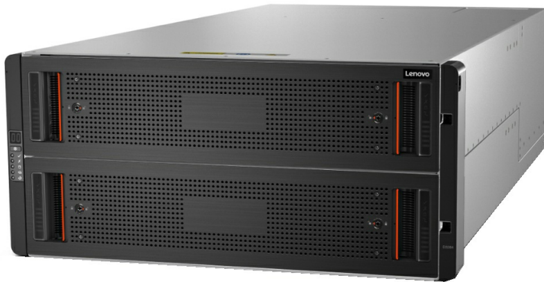
Figure 4. Lenovo Storage D3284 External High Density Drive Expansion Enclosure
