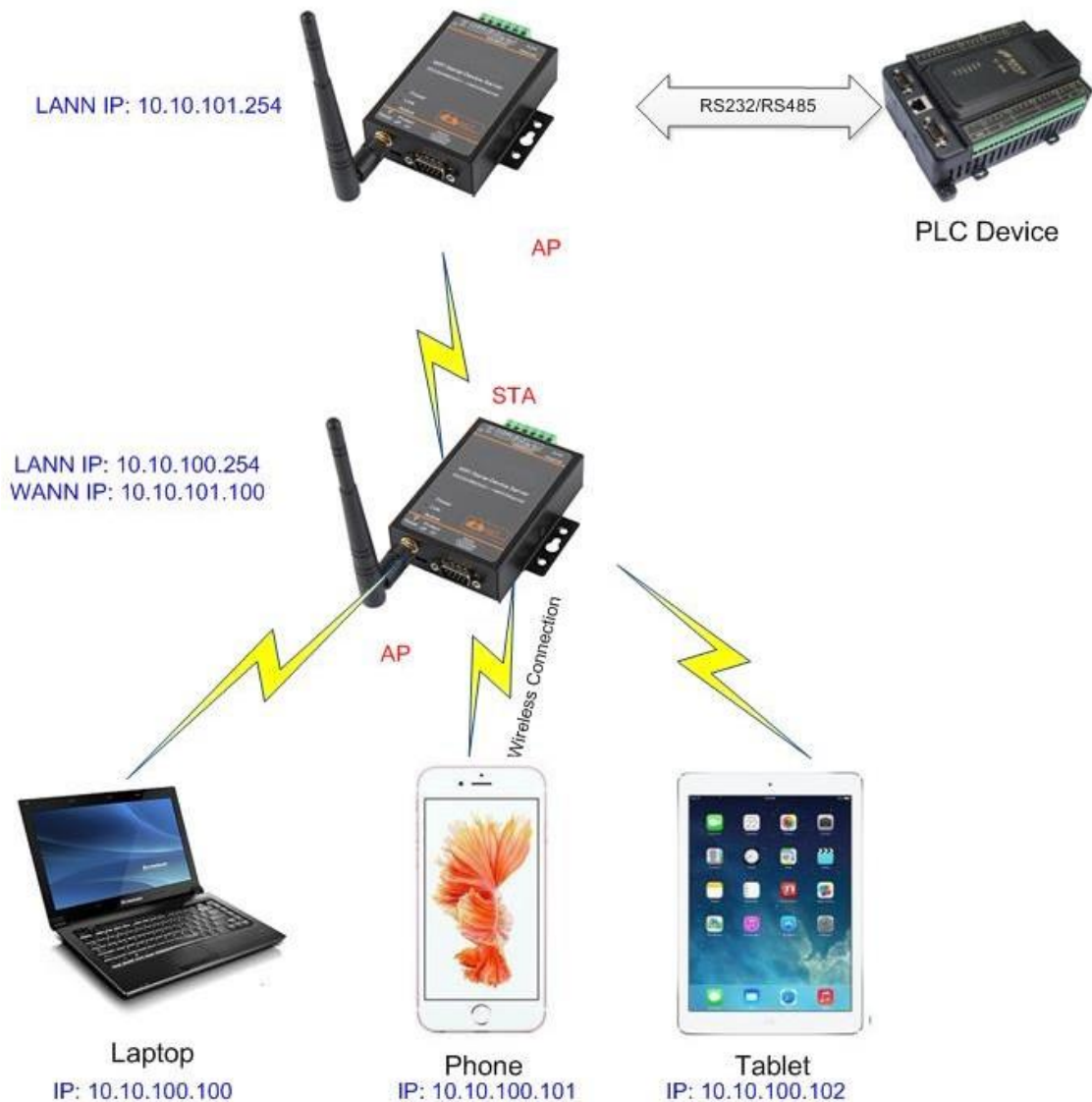
Figure 14. AP+STA Wireless Network
