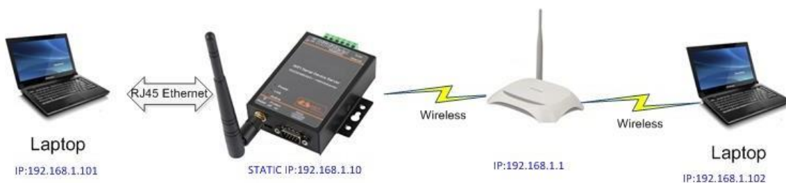
Figure 22. Ethernet Port Function (Bridge)
