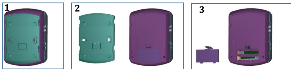
Figure 9. Steps for disassembling device for batteries replacement
