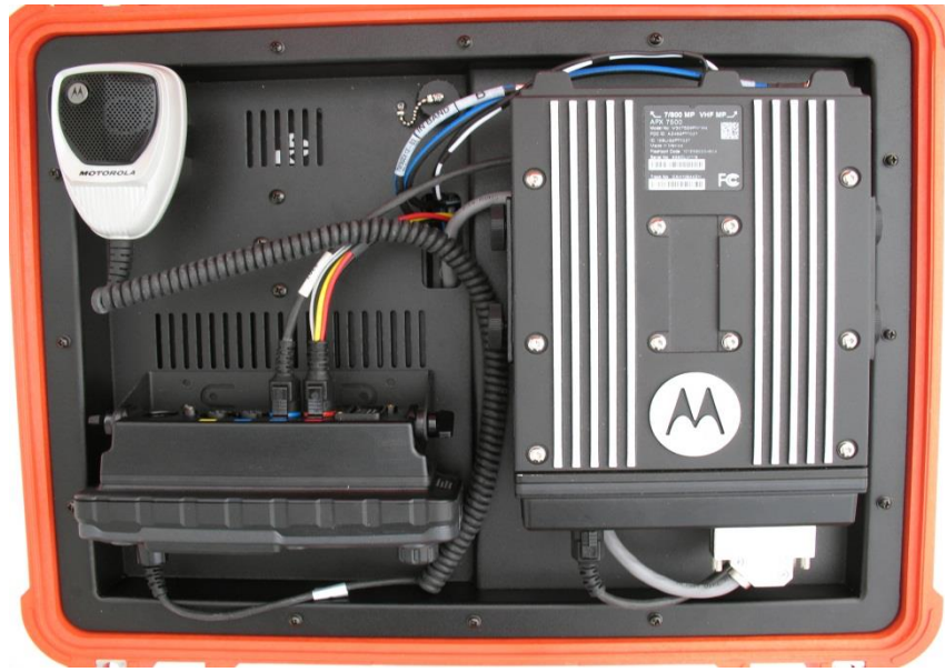
Figure 11 Fully Assembled Suitcase Mount DVRS O2 Control Head Models
