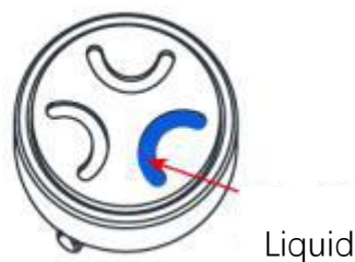
Figure 2-5-2 Dead volume (Sealed rotor)
