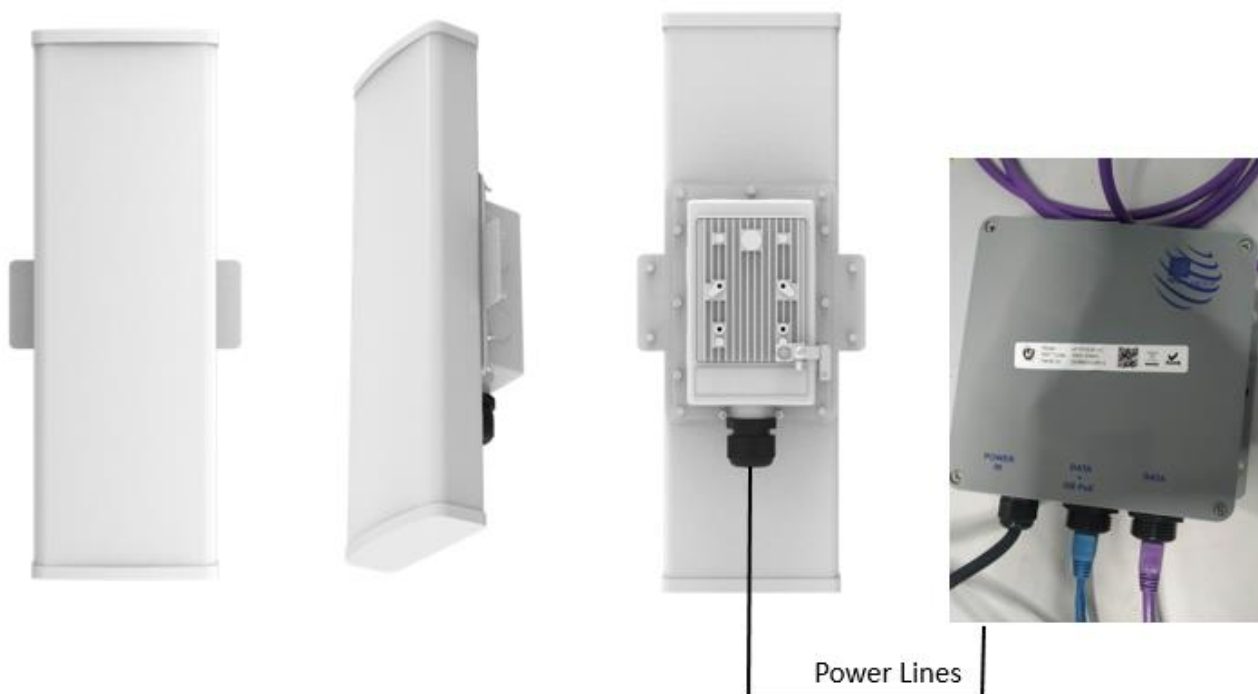
Figure 3: Power up the Outdoor device of 17dB Sector Antenna using Active PoE adaptor
