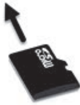
Figure 2. Insert microSD card into new controller
