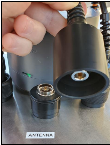
Figure 4 & 5: Iridium RF cable antenna connected to X2 antenna port.
