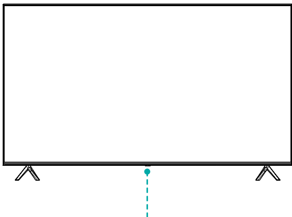
Remote sensor / Power indicator / Single button (Standby / Source)
