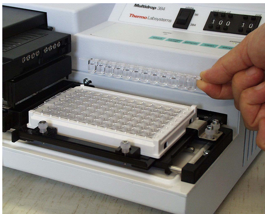
Fig. 7.9 Removing the filled microstrip to be weighed
