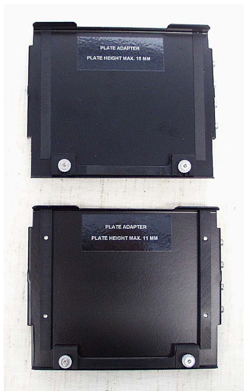
Fig. 6.7 Two different plate adapters
