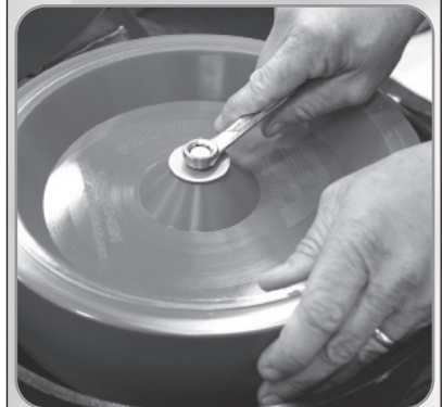
Figure 7 Hold wheel in place while loosening bolts.
