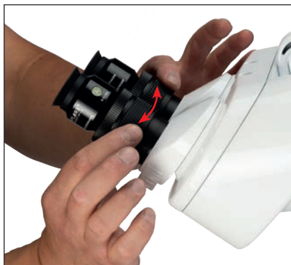
17. Focusing by means of helical single focusing.
