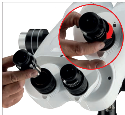
16. Insert and clamp the eyepieces.
