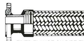
FIXED FLANGE ON PIPE END
