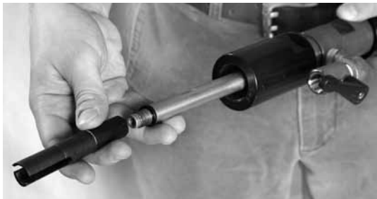
Attach coupling nut to shell cutter.
