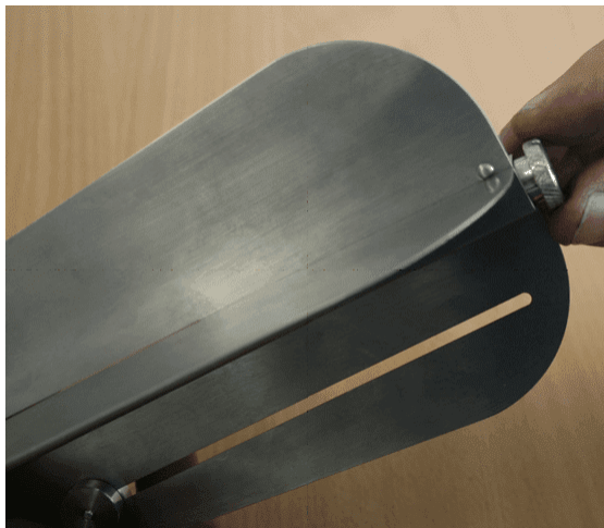
Step5. Ensure the adaptor is jammed tight against the tail pieces
