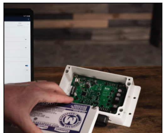
Figure 2 - Removing the regulator lid
