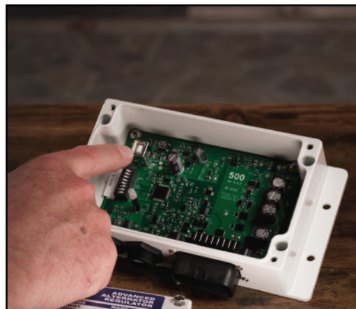
Figure 5 - Type B USB connector & reset button
