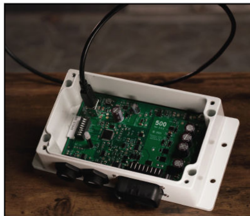
Figure 6 - Type B USB cable connected
