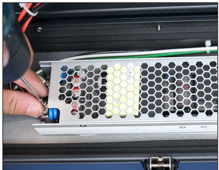
Figure 48: Remove Hardware from Power Supply
