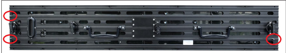
Figure 34: Connector & Locator Pins on Module Rear
