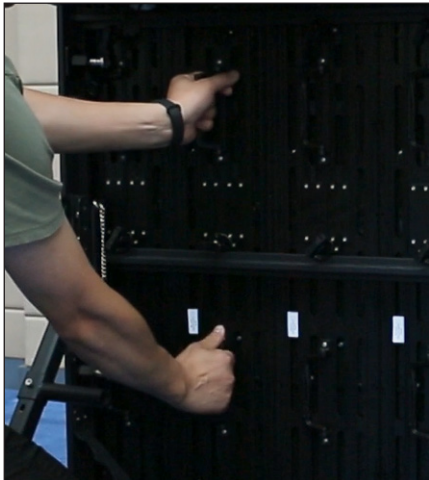
Figure 32: Grasp Handles on Rear of Module
