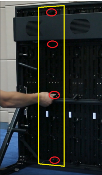
Figure 29: Unlock Module Latches
