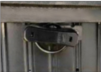
Figure 31: Unlocked Module Latch Position
