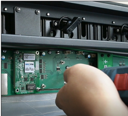
Figure 36: Remove Screws Securing Receiver Card to Hub Board
