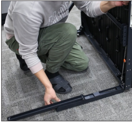
Figure 19: Fold Stiffener Down into Foot Structure
