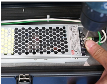
Figure 47: Remove Cables from Power Supply
