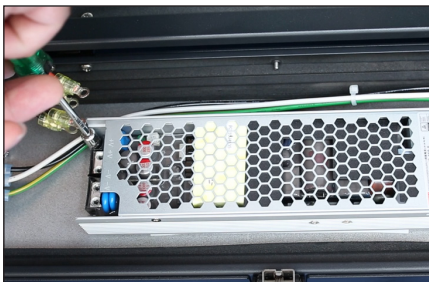
Figure 49: Remove Nuts from Power Supply
