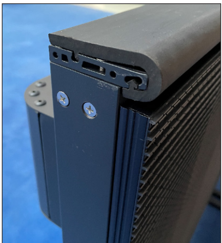
Figure 52: Top Pad Seated Properly
