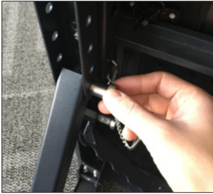
Figure 18: Remove Locking Pin from Stiffener
