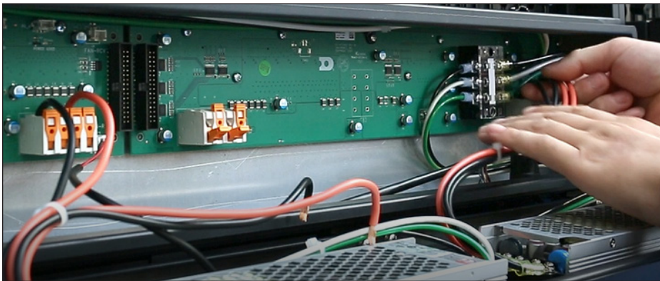
Figure 41: Disconnect Power & Signal Cables from Hub Board
