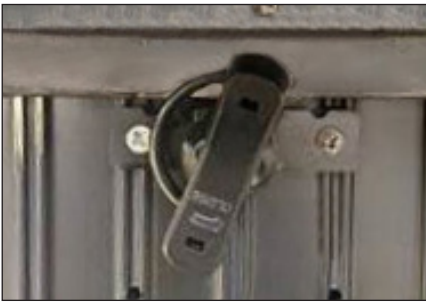
Figure 30: Fully Locked Module Latch Position
