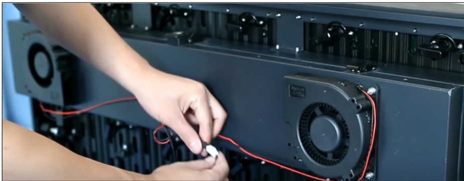
Figure 44: Disconnect Fan Cable from Connector
