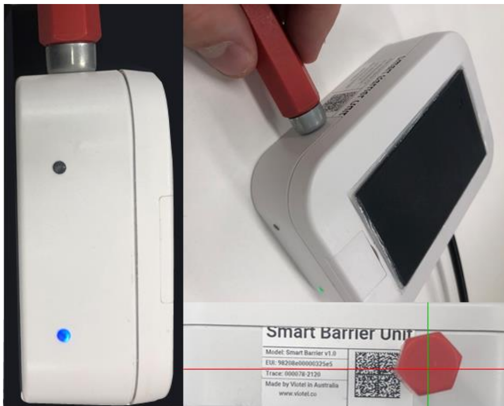
Figure 2 Magnetic Key Location
