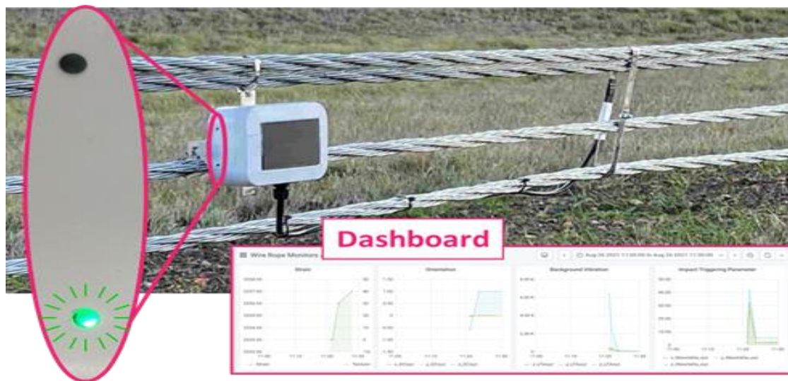
Figure 3 LED Location and Dashboard Data
