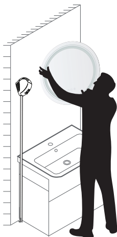
1.Measure the best installation height with a tape measure
