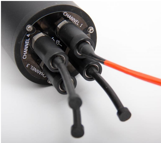
Figure 1: Four channel FDL Mini seen from the sensor connector end. An In Situ UniAmp amplifier is plugged into channel 1 and channels 2-4 are closed with dummy plugs.
