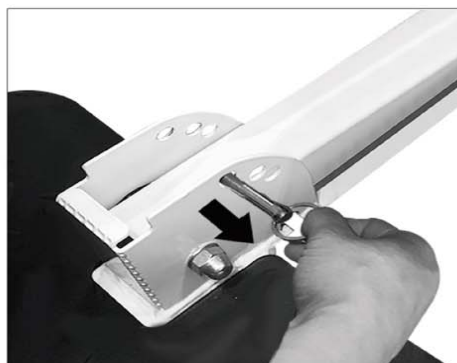
2 Pull out the bolt
