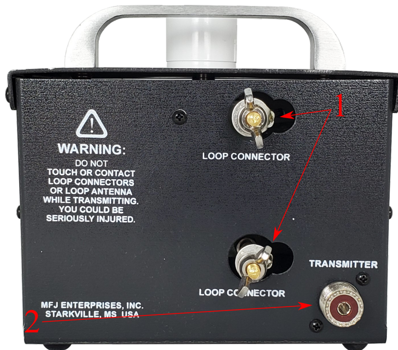
Figure 5: Rear-panel Connections: 1.) Wire loop connectors, 2.) Coax input
