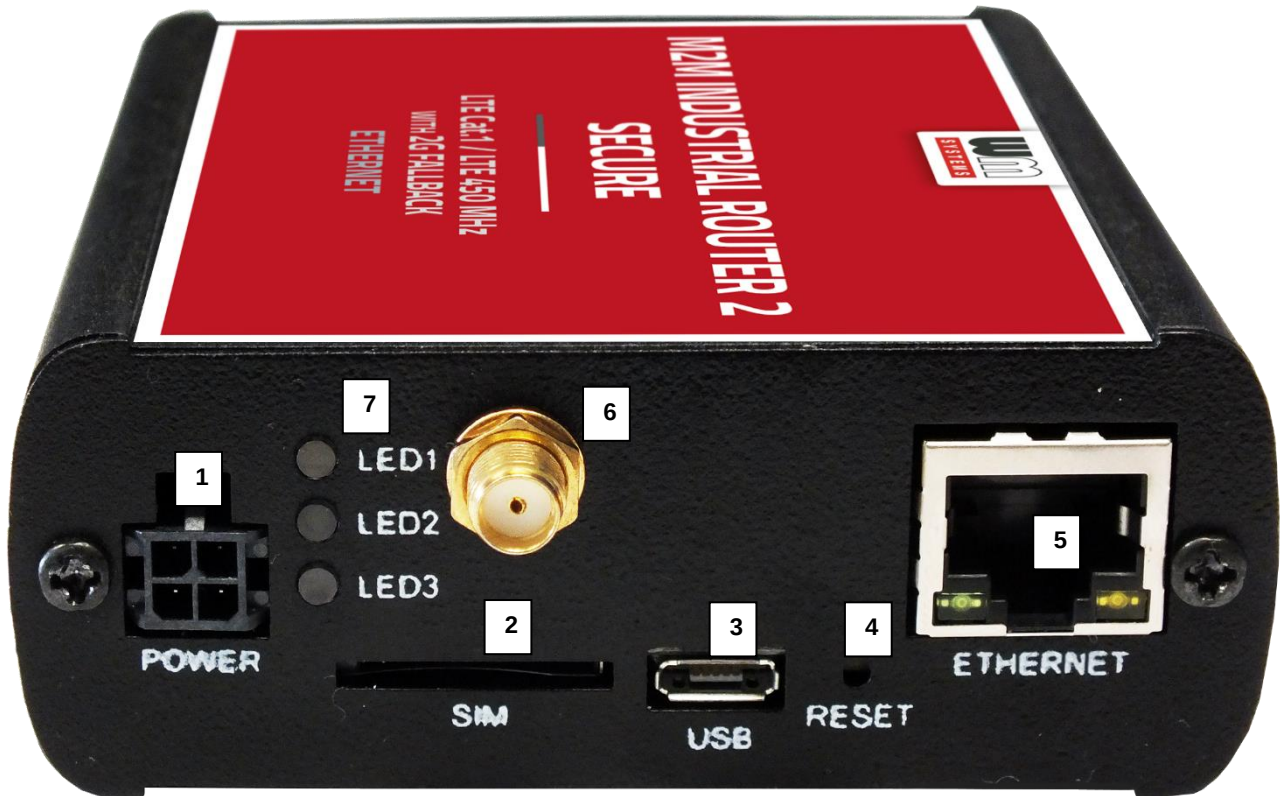
Industrial secure router, assembled in aluminum casing with interface connectors / ports
