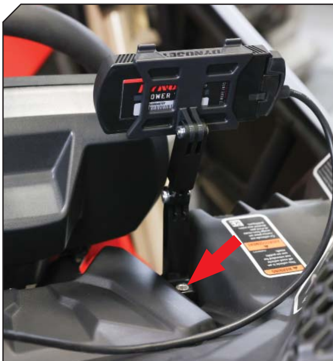
INSTALL BASE AND CLAW MOUNT
