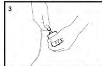
Connect end of pump connection to adapter
