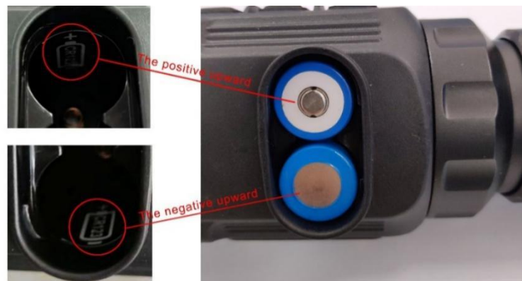
Fig. 8-1 Schematic diagram of battery installation
