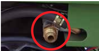
Gas Inlet (Figure B) Propane / NG
